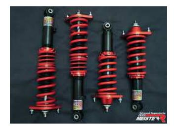
talk to them explaining your style of driving. I had a set on my '06 but I went to a slightly softer spring rate for a more comfortable ride. Spring rate is listed as the force it takes to compress the spring a set distance. These came with 7kg front springs and 5kg rear. I changed to 6kg front and 4kg rear for a compromise of better ride vs. handling.
