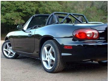
To fix what I considered the only major shortfall of the Miata, I installed a supercharger that put 175 HP and 150ft lbs of torque to the rear wheels. Along with some additional handling upgrades, it was a fantastic car. It had great power and handling and along with the other qualities of the Miata, a near perfect car.
