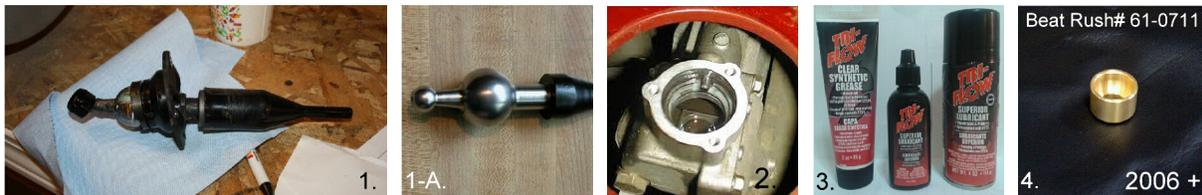
Grease on the large ball can help keep the shifter working smoothly. The round ball in the center is metal, and it rotates inside 2 plastic “rings”. You can see a glimpse of the narrow gray ring resting on the top of the ball in picture 1. There is another one (white ring) down inside the turret in picture 2.
