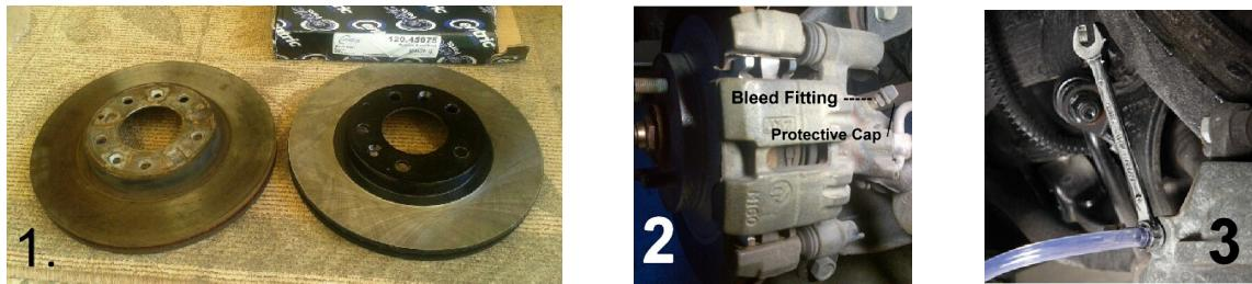
The easiest way to flush new fluid is to remove one wheel at a time to gain access to the bleed fitting on each caliper as in picture # 2. Remove the rubber cap, put a small wrench on the fitting and attach a hose to the fitting as in picture # 3. Put the other end of the hose into a bottle as in picture #4.
