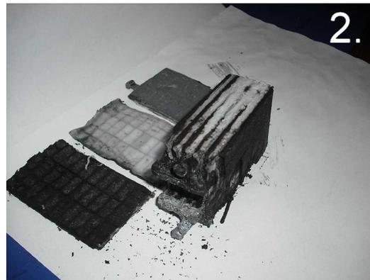
The earlier NA and NB series Miatas up to 2005 use a somewhat sealed battery called a AGM or “Absorbed Glass Mat” battery. The battery works like the lead acid battery explained above, but the acid is absorbed between the lead plates by a very fine fiberglass mat. See picture #2. This glass mat absorbs and immobilizes the acid while still keeping the acid available to the plates. This allows a fast reaction between acid and plate material.
