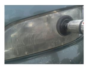
The picture below Left is during the 2nd polishing step. I put some of the polishing compound on the thicker polishing pad, kept a little water on the lens, and moved the pad all around on the lens surface. This 2<sup>nd</sup> step is to remove any scratches that may be in the lens surface and polished it like new. You can see in the picture below Right how well it restored the car's headlight lens to a very clear state!
