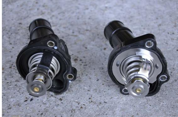
You can NOT tell if you have this problem by watching the Temp Gage in the dash. This gage does not totally show the coolant temps. The coolant should run about 185 degrees at normal operating temperature. The gage stops moving upwards at 158 degrees. Why?? Who knows?? The gage only goes higher if you have an overheating problem.
