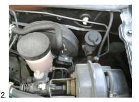
The picture #2 above RIGHT shows BOTH the Brake and Clutch fluid reservoirs for up to year 2005 Miatas. In this picture above right you will see the power brake booster tank and brake master cylinder & reservoir on the left side, and the clutch master cylinder has the little reservoir on the right side with the black cap. Be sure to keep them both filled with the proper fluid.
