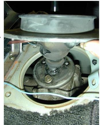
The easiest way to remove the small boot is to put the tranny in neutral and just pull the shifter straight up and out of the tranny. Before you pull the shaft up out of the tranny,
