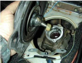
First you must unscrew the shifter knob. It is probably tight, but just turn it to the left and it will come off. Then remove the console. There will be screws hidden in the storage box section, under the cup holders, and even under the (NB) electric window switches.
