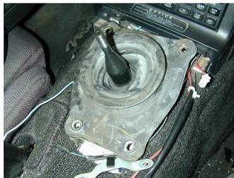
put a mark on it facing you so you put it back in the same way. You should see a small plastic "cup" type bushing on the bottom end of the shifter. (See attached picture of plastic bushing) If you have a 1989 to 2005, 5 speed tranny, now would be a good time to suction the lube out of the top turret section and put new oil in. (1989 to 2005 6-speed
