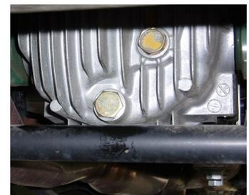
Big chunks mean a problem. Install the drain plug and fill the Diff until oil runs out the fill plug, Then secure the fill plug. Carefully lower the car to the ground, and enjoy.
