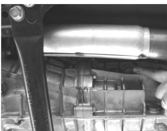
The fill plug in all of the manual trannies (89 to present) is always on the driver’s side of the tranny. (See attached picture) It is a square head pipe plug, just like you would use in home plumbing. DO NOT remove any bolts on the passenger’s side of the tranny. These hold internal parts in place. Always be sure to remove the fill plug first, especially if it has been many years since it has been changed as it
