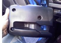
sheet metal screw type threads. The 3rd screw is a metal fine thread type screw closest to the dash. If you have the advanced Keyless Entry, and have the plastic knob in the ignition switch like in the picture, remove this plastic knob first as it
