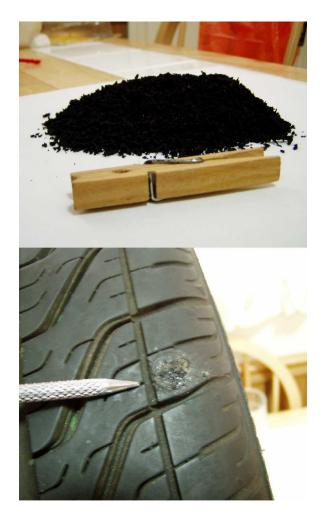
The last picture top section has a pile of rubber that came out from inside my tire. The pile was bigger around and taller than the clothespin lying in front of it. A surprising amount as I only drove about 100 yards after I picked up the large screw. The bottom part of this picture shows the outside of the tire where I trimmed the plug. It is a gummy mess to trim, so you can't make it perfect. But if I would have driven on it a while, it would have worn smooth.
